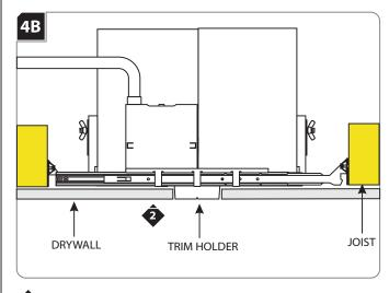
2 Align the cut out section of drywall with the trim holder and install drywall.
