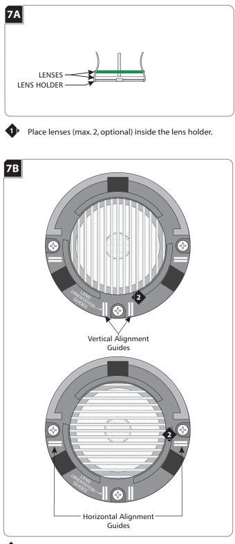
• Use the lens orientation guides to align linear spread lenses vertically or horizontally.
