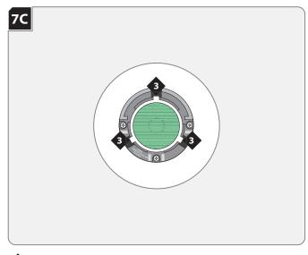
Line up the legs of the lens holder with the notches on the lamp holder and push the lens holder on.
