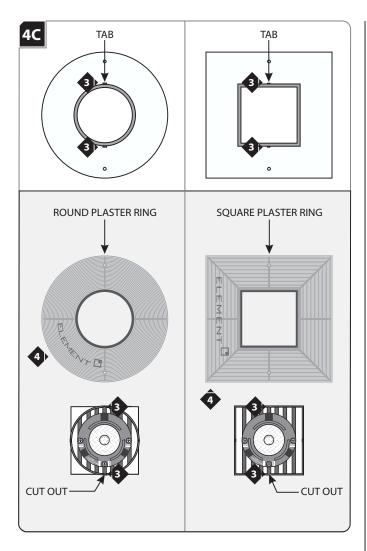
3 Line up the two tabs in back of the plaster ring with the two cut out sections of the trim holder inside edge.
