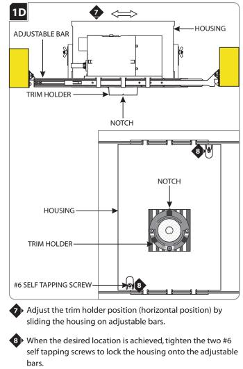
**NOTE:** Notches in trim holder can be used to align multiple housings using a laser or string.
