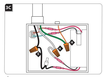
Connect the neutral power line wire to the white transformer wire with a wire nut.
