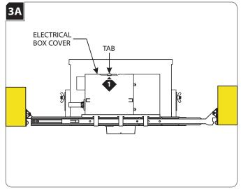
Push the tab on the housing electrical box up and remove the electrical box cover.
