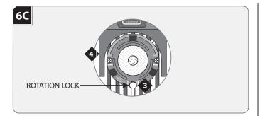
**NOTE:** Lamp housing can rotate 361° horizontally.
