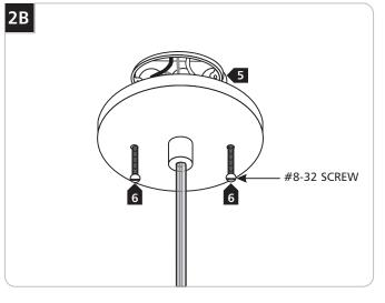
5 Place all wires, wire nut connections, and the driver properly inside the canopy.
