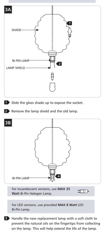
4 Gently insert the new lamp into the socket.
