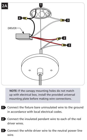
4 Connect the black driver wire to the hot power line wire.
