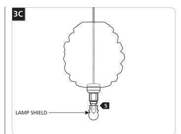
**5** Push the lamp shield onto the spring clip.
