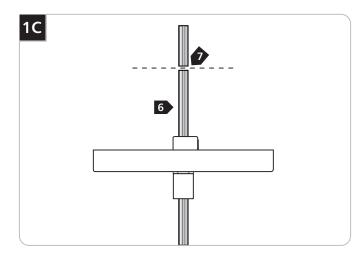
6 For power connection, leave at least 6" of the cord exposed in the back of the canopy.
