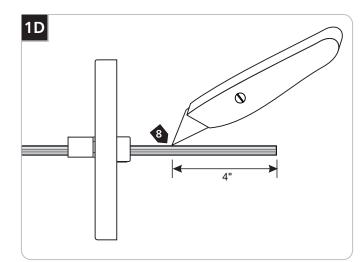
8 From the end of the cord, strip the outer insulation 4" using a sharp knife and needlenose pliers. Make sure not to cut inner wires.
