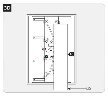
6 Replace the lid onto the center housing and tighten the screws.
