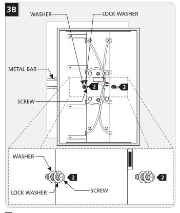
2 Mount the pan to the metal bar with the washers, lock washers and screws provided.
