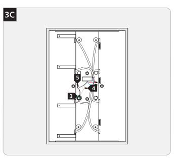
Connect the fixture to a suitable ground in accordance with local electrical codes.
