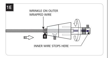
6 Keep pushing the coaxial cable into the connector while rotating the connector to ease feeding the inner wire into the tip of the connector. The outer wrapped wire will start wrinkling while being inserted another 1/2" into the connector.
