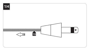
10 Pull the coaxial cable toward the fixture to smooth the wrinkles.
