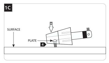
4 Tap the conical connector on a hard surface with the set screw facing down, so the plate inside drops into place.
