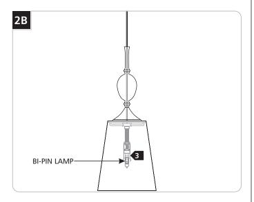
For incandescent versions, use MAX 50 Watt Bi-Pin Halogen Lamp.
