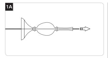
1 Feed the coaxial cable through the glass fount.
