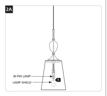
1 Remove the lamp shield and the old lamp.
