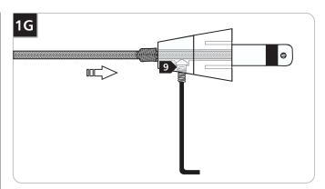
**9** Firmly tighten the set screw on the conical connector.
