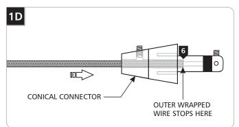
6 Feed and push the coaxial cable into the conical connector. The coaxial cable will come to a stop point after being inserted 3/4" into the conical connector.
