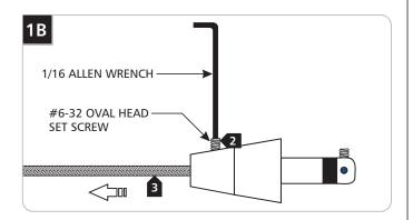
2 Back out (do not remove) the #6-32 oval head set screw on the conical connector with the provided 1/16 Allen wrench.
