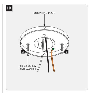
Secure the mounting plate to the electrical box with the two #8-32 screws provided.
