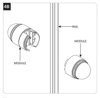
2 Install the two module halves onto the rail and secure in place by screwing them together. Make sure to match the polarity markings positive (+) and negative (-) on the rail.
