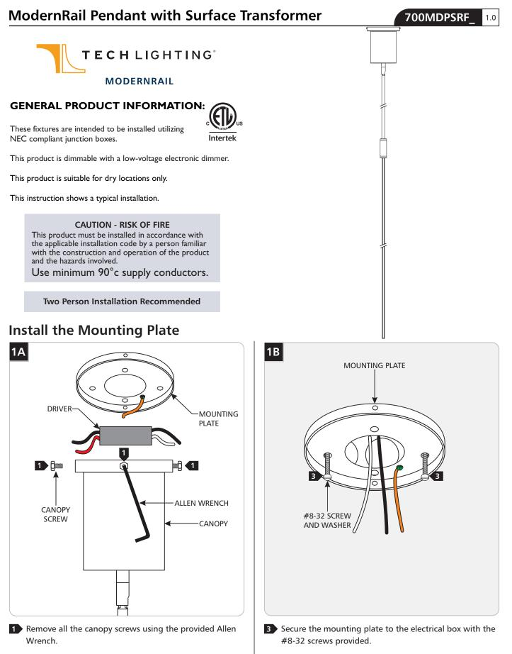
2 Remove the mounting plate and driver from the canopy.
