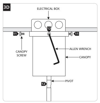
10 Neatly place all wires and wire nut connections inside the canopy.
