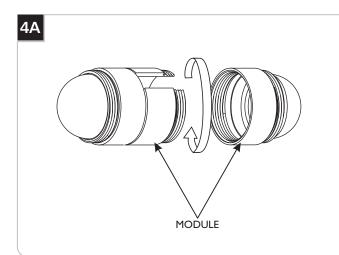
Separate the two halves of the module by unscrewing them from one another.
