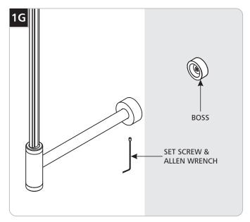
Place the lower arm onto the boss and secure them together by screwing in the set screw using the provided Allen wrench.
