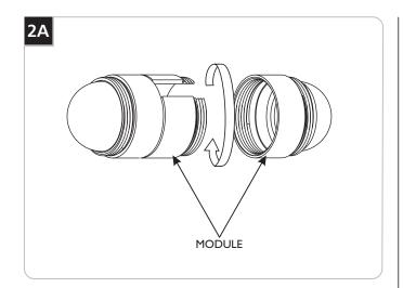
1 Separate the two halves of the module by unscrewing them from one another.
