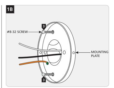
Secure the mounting plate to the electrical box with the #8-32 screws provided.
