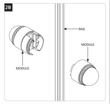
Install the two module halves onto the rail and secure in place by screwing them together. Make sure to match the polarity markings positive (+) and negative (-) on the rail.
