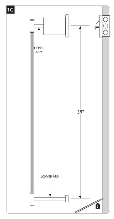
4 Using the diagram above, mark the anchor hole location for the lower arm onto the wall. The fixture measure 39" from the center of the upper arm to the center of the lower arm.
