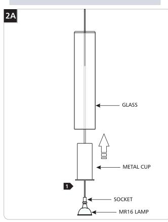
1 Move the fixture glass and metal cup up to expose the socket.
