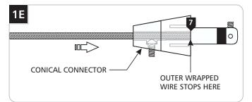
Feed and push the coaxial cable into the conical connector. The coaxial cable will come to a stop point after being inserted 3/4" into the conical connector.
