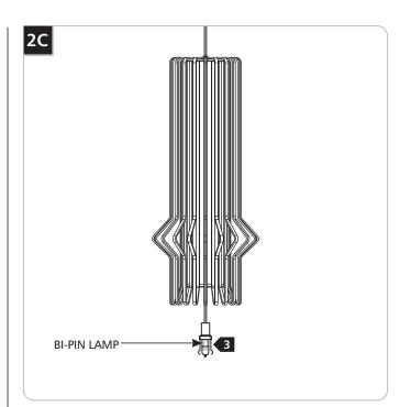
**NOTE: For halogen versions only**, handle the new replacement lamp with a soft cloth to prevent the natural oils on the fingertips from collecting on the lamp. This will help extend the life of the lamp.
