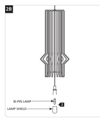
2 Remove the lamp shield and the old lamp.
