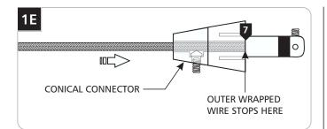
Feed and push the coaxial cable into the conical connector. The coaxial cable will come to a stop point after being inserted 3/4" into the conical connector.
