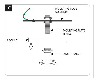
Separate the mounting plate assembly from the canopy by unscrewing the hang straight from the mounting plate nipple.
