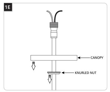
Unscrew the knurled nut downward until it is completely un-threaded and carefully slide it down the stem, followed by the fixture canopy.
