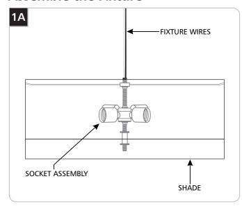
1 Feed the fixture power line through the shade's center ring and install the shade onto the socket assembly.
