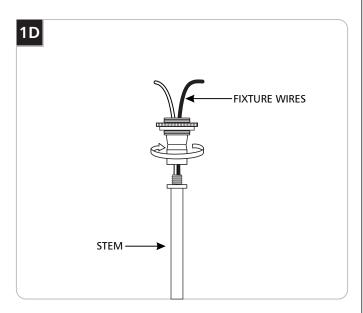
4 Feed the fixture wire through the hang straight and screw it securely onto the stem.
