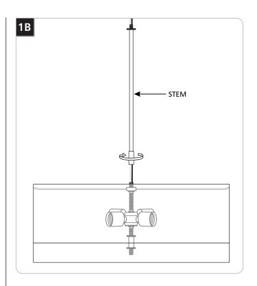
**2** Feed the fixture wires through the stem and screw the stem completely onto the socket assembly.
