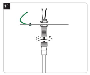
Feed the fixture wires through the center of the threaded nipple on the mounting plate assembly and screw it completely into the hang straight. Make sure the crossbar is securely tightened.
