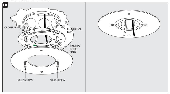
**NOTE:** The crossbar or mounting plate may vary depending on the fixture. Follow the fixture's installation instructions for any additional steps that may be needed to proper install the crossbar/mounting plate.
