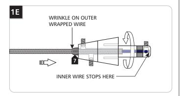
7 Keep pushing the coaxial cable into the connector while rotating the connector to ease feeding the inner wire into the tip of the connector. The outer wrapped wire will start wrinkling while being inserted another 1/2" into the connector.
