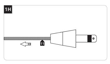
11 Pull the coaxial cable toward the fixture to smooth the wrinkles.
