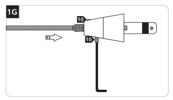
10 Firmly tighten the set screws on the conical connector.
