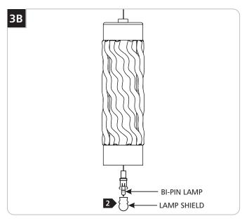
2 Remove the lamp shield and the old lamp.
