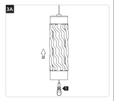
1 Lift the glass shades up to expose the socket.
