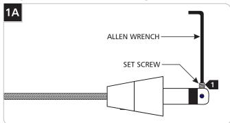
Back out (do not remove) the set screw on tip of the connector with the provided Allen wrench.
