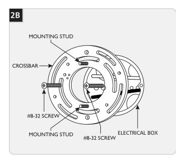
2 Align the two mounting studs vertically and mount the crossbar to the electrical box with the two #8-32 screws provided.
