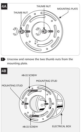
2 Align the two mounting studs horizontally and mount the crossbar to the electrical box with the two #8-32 screws provided.
