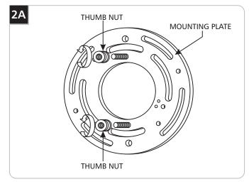
Unscrew and remove the two thumb nuts from the mounting plate.
