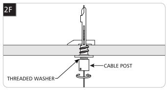
Tightly screw the cable post back onto the threaded washer.
