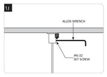
Ensure that the set screws in both the canopy and the cable post are tight with the provided Allen wrench.
