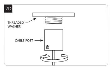
5 Unscrew the threaded washer to separate it from the cable post.
