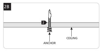
Tap one of the anchors at the marked point into the wall up to the threaded portion with a hammer.
