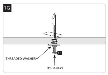
15 Screw the threaded washer onto the anchor with the long #8 screw.
