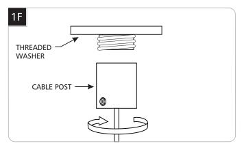
14 Unscrew the threaded washer to separate it from the cable post.
