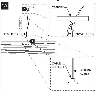
**NOTE**: The power cord does not support the fixture. For a casual "lazy cord" look, cut the power cord several inches longer than the drop height of the fixture.
