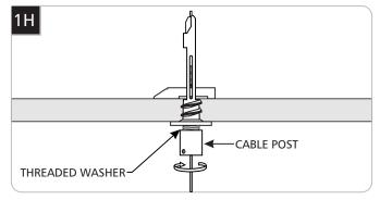
**16** Tightly screw the cable post back onto the threaded washer.
