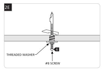
6 Screw the threaded washer onto the anchor with the long #8 screw.
