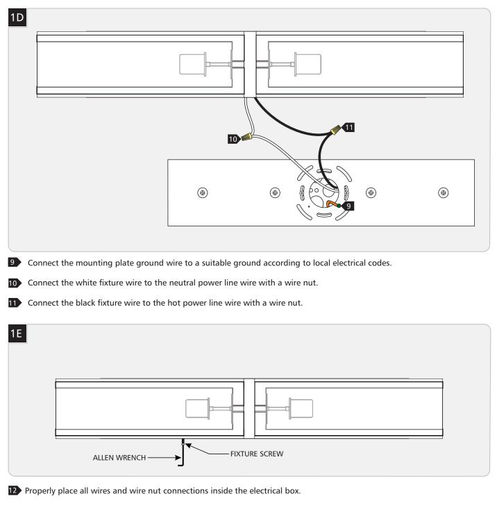
B Re-place the fixture onto the backplate and re-install the fixture screws.
