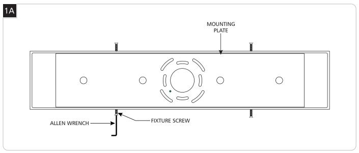
With the Allen wrench provided, unscrew and remove the four fixture screws.
