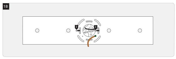
3 Level the mounting plate and secure it to the electrical box with the two #8-32 screws provided.
