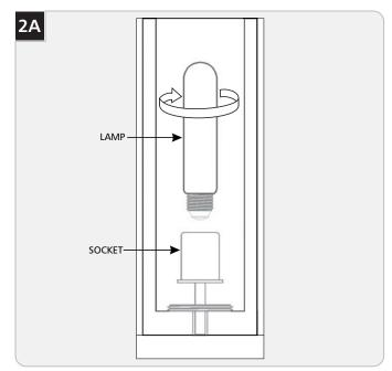
**CAUTION:** To reduce the risk of a burn or electric shock during relamping, disconnect the power to the fixture.
