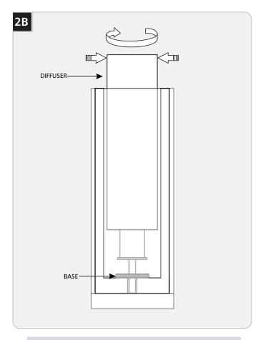
**CAUTION:** When installing the diffuser, apply even pressure on each side of the diffuser by using both hands to screw it in place. **DO NOT OVER TIGHTEN** the diffuser. This may break the glass resulting in injury.
