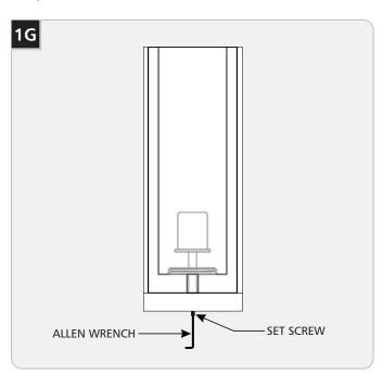
14 With the allen wrench, tighten the set screw at the bottom of the fixture to secure it to the mounting plate.
