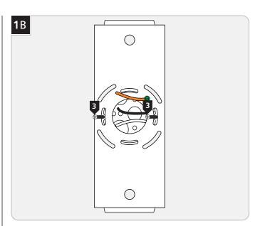
Level the mounting plate and secure it to the electrical box with the two #8-32 screws provided.
