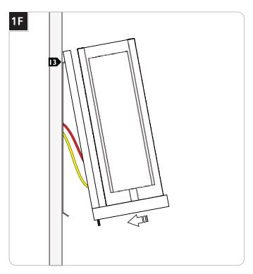
Hook the top of the fixture to the top of the mounting plate and swing the bottom of the fixture toward the plate until it is flush with the wall.
