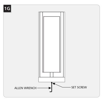
14 With the allen wrench, tighten the set screw at the bottom of the fixture to secure it to the mounting plate.
