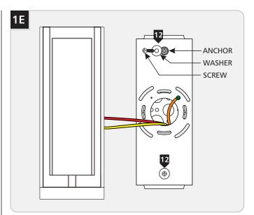
12 Slide a #8 screw through a washer, and screw it into an anchor to secure the fixture base to the wall. Repeat for the other anchor.
