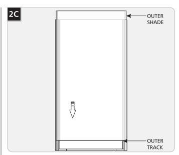
Gently slide the edges of the outer shade down the outer tracks in the fixture base until it rests against the end of the tracks.
