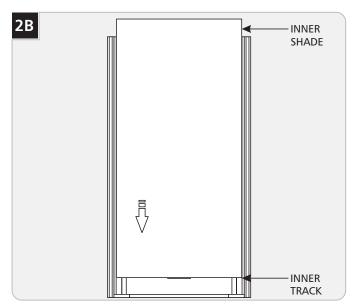
2 Gently slide the edges of the inner shade down the tracks in the fixture base until it rests against the end of the inner tracks.
