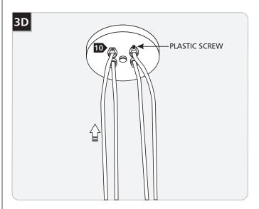
10 Push the excess power feed wires into the canopy and tighten the plastic screws.
