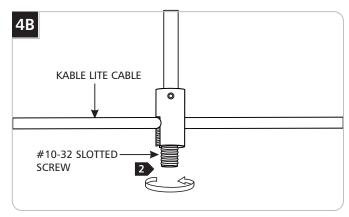
2 Place the power feed connectors onto each Kable Lite cable. Replace and tighten the #8-32 slotted set screw.
