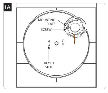
Remove the mounting plate from the top of the fixture base by rotating the screw heads out of the keyed slots.
