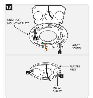
Depending on the electrical box, use one of the following methods to install the #8-32 screws:
