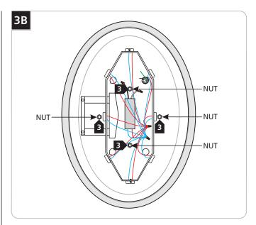
Tighten the four provided nuts to secure the pan onto the backplate.
