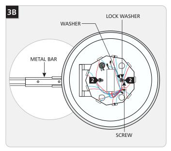
2 Mount the pan to the metal bar with provided washers, lock washers and the screws.
