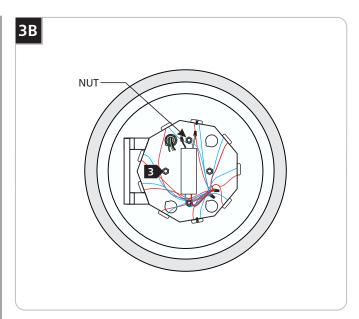
Tighten the four provided nuts to secure the pan onto the back plate.
