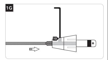
Tighten the #6-32 oval head set screw on the conical connector firmly.
