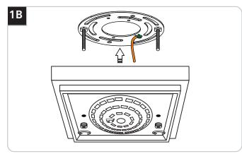
Remove the mounting plate from the fixture base by unscrewing the two knurled nuts.
