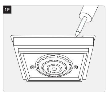
**9** For wet location installation, caulk around the fixture base with waterproof construction sealant.
