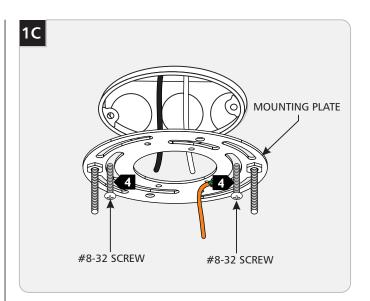
Secure the mounting plate to the electrical box with 2 #8-32 screws.
