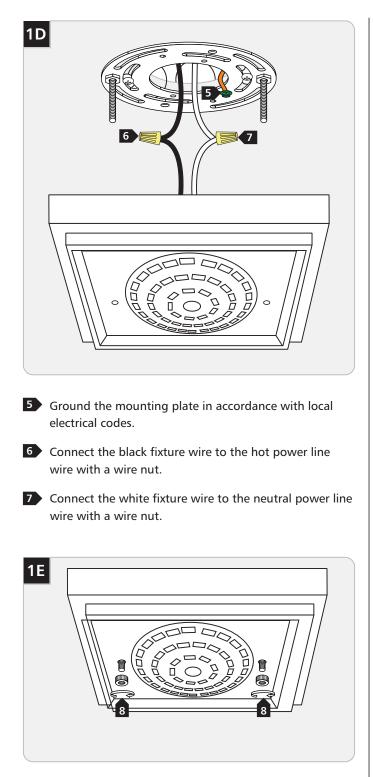
Properly place all wires and wire nut connections into the electrical box, mount the fixture base to the ceiling by reinstalling it onto the mounting plate, and secure it tightly with the knurled nuts.
