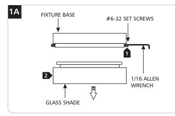
While supporting the glass shade, loosen (**Do Not Remove**) the four #6-32 set screws on fixture base with the 1/16 Allen wrench.
