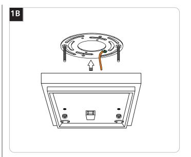
Remove the mounting plate from the assembly by unscrewing the two knurled nuts.
