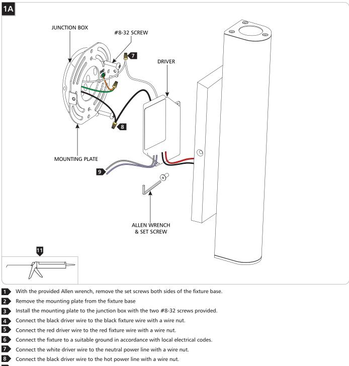
**9** For 0-10V Dimming Only: Connect the purple and gray wires to a compatible dimmer. If not using 0-10V dimming, cap off the purple and gray wires.
