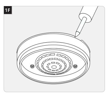
**For wet location installation**, caulk around the fixture base with waterproof construction sealant.
