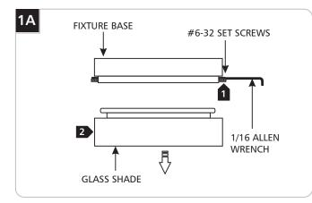
While supporting the glass shade, loosen (Do Not Remove) all the #6-32 set screws on fixture base with the 1/16 Allen wrench.
