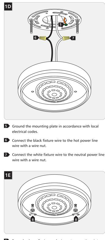
Properly place all wires and wire nut connections into the electrical box, mount the fixture base to the ceiling by reinstalling it onto the mounting plate, and secure it tightly with the knurled nuts.
