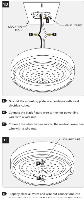
Properly place all wires and wire nut connections into the electrical box, mount the fixture base to the ceiling by reinstalling it onto the mounting plate, and secure it tightly with the knurled nuts. 1F
