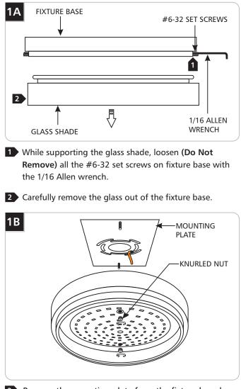
Remove the mounting plate from the fixture base by unscrewing the two knurled nuts.
