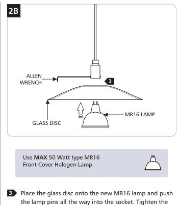
bottom two set screws with the Allen wrench.
