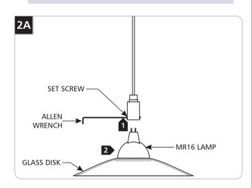
Hold the glass disk and lamp with one hand and loosen (Do Not Remove) the bottom two set screws with the provided Allen wrench.
