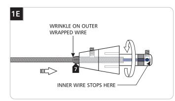
Keep pushing the coaxial cable into the connector while rotating the connector to ease feeding the inner wire into the tip of the connector. The outer wrapped wire will start wrinkling while being inserted another 1/2" into the connector.
