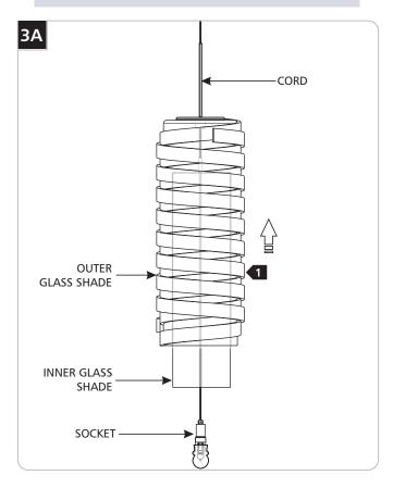
1 Carefully lift the glass shades up to expose the socket.
