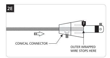
7 Feed and push the coaxial cable into the conical connector. The coaxial cable will come to a stop point after being inserted 3/4" into the conical connector.
