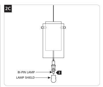
Remove the lamp shield and the old lamp.
