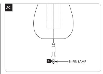
For incandescent versions, use MAX 35 Watt Bi-Pin Halogen Lamp.
