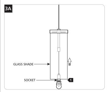
1 Lift the glass shade up to expose the socket.
