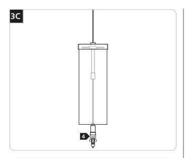
For incandescent versions, use MAX 50 Watt Bi-Pin Halogen Lamp.
