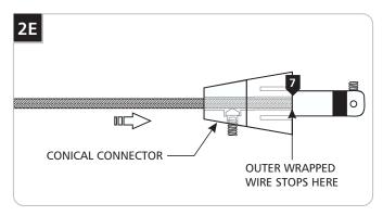
7 Feed and push the coaxial cable into the conical connector. The coaxial cable will come to a stop point after being inserted 3/4" into the conical connector.
