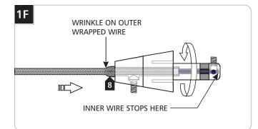
8 Keep pushing the coaxial cable into the connector while rotating the connector to ease feeding the inner wire into the tip of the connector. The outer wrapped wire will start wrinkling while being inserted another 1/2" into the connector.
