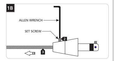
2 Back out (do not remove) the set screw on the conical connector with the provided Allen wrench.
