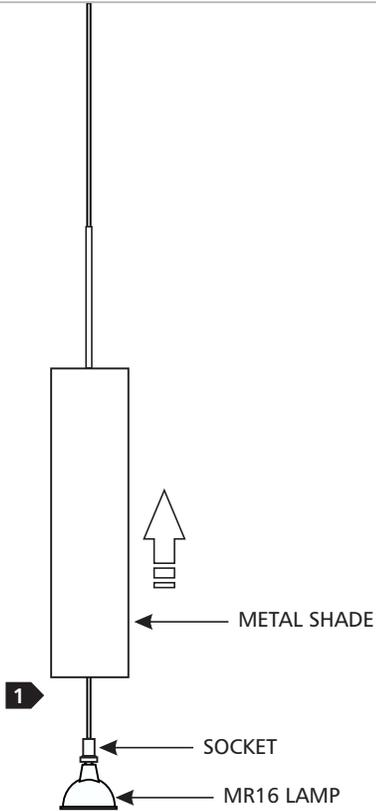
**1** Move the fixture metal shade up to expose the socket.
