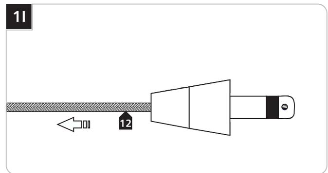
**12** Pull the coaxial cable toward the fixture to smooth the wrinkles.
