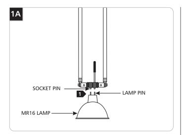
Use **MAX** 75 Watt, MR16 Front Cover Halogen Lamp.
