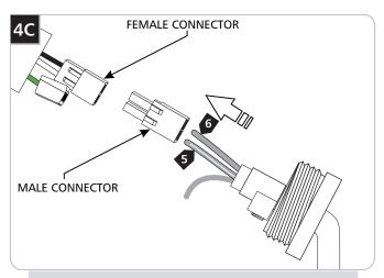
**CAUTION:** Exposed hot and neutral conductors may result in a short. Ensure no bare wire is exposed.
