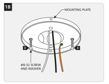
3 Secure the mounting plate to the electrical box with the two washers and #8-32 screws provided.
