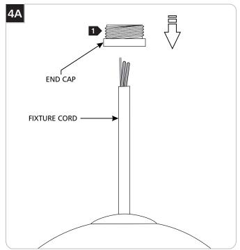
1 Slide the end cap over the fixture cord making sure the threading faces upward.
