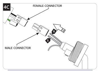
**CAUTION:** Exposed hot and neutral conductors may result in a short. Ensure no bare wire is exposed.
