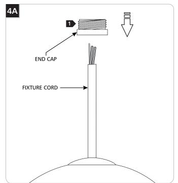
1 Slide the end cap over the fixture cord making sure the threading faces upward.
