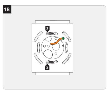
Attach the mounting plate to the electrical box using the two provided #8-32 screws.
