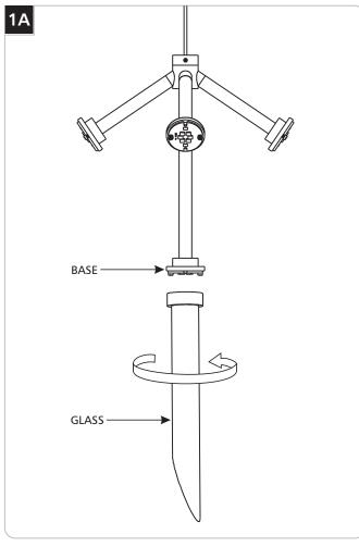
Install the glass by screwing it into the base. Do not over-tighten.
