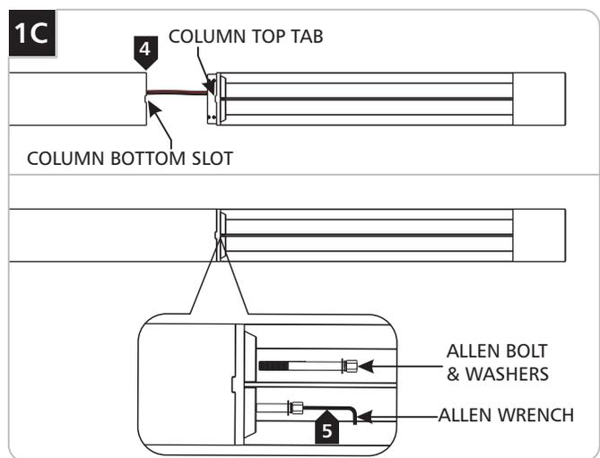
**4** Align the tab on the column top to the slot in the column base, insert the fixture wires into the column base, and assemble them together.
