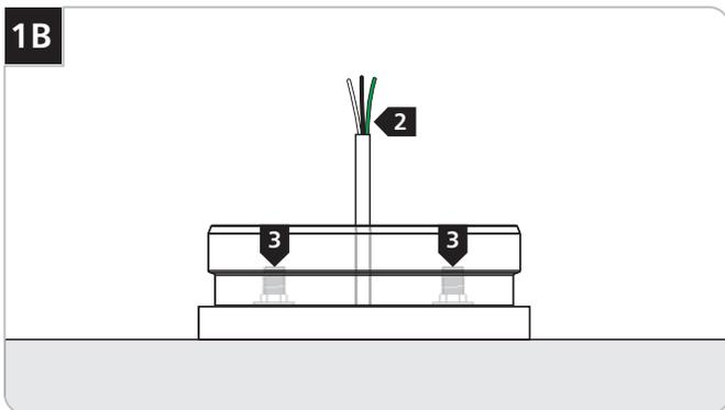
**2** Bring the power wires to the fixture location in accordance with local electrical codes.
