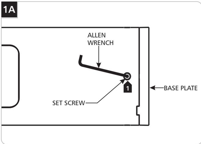
**1** Loosen (**Do Not Remove**) the four set screws on column base with the provided Allen wrench and remove the base plate.
