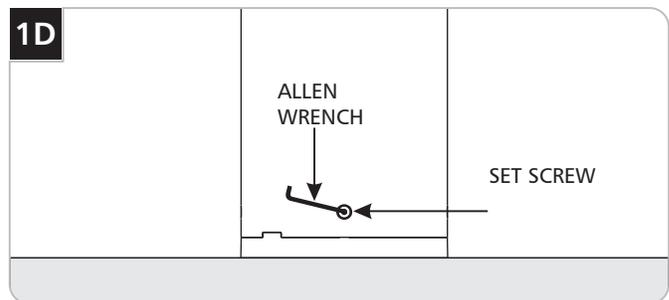
**6** Carefully install the column assembly onto the base plate and secure it in place by tightening all 4 set screws.
