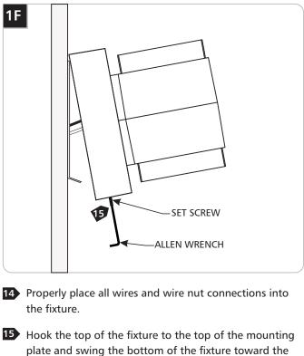
plate and swing the bottom of the fixture toward the plate until it is flush with the wall.
