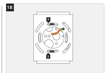
Attach the mounting plate to the electrical box using the two provided #8-32 screws .
