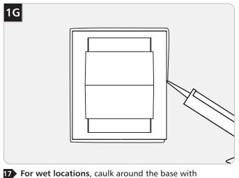
For wet locations, caulk around the base wit waterproof construction sealant.
