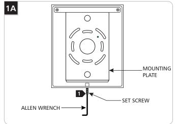
With the Allen wrench provided, back out (do not fully remove) the set screw at the base of the fixture.
