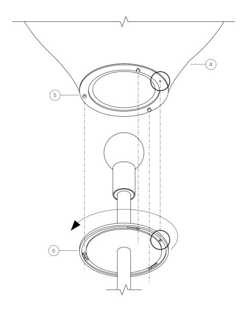
Tighten the pin  $\bigodot$  and arrest the closed position.
