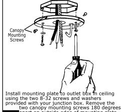
two canopy mounting screws 180 degrees apart on outside edge of mounting plate.
