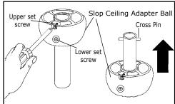
**Warning**: Cross pin must be installed in the slot of Slop ceiling adapter ball and through downrod.
