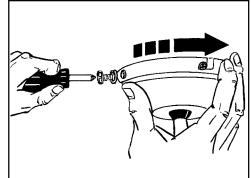
Rotate canopy clockwise until both mounting screws drop into slot recesses. Tighten screws securely. Install third and fourth screws with lockwashers into mating holes and tighten.
