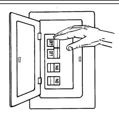
Turn off power at breaker box to avoid possible electrical shock.
