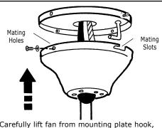
Carefully lift fan from mounting plate hook, making sure not to break any wire connections. The canopy has (2) mating slots and (2) mating holes (see illustration above). Position both slots in canopy directly with (2) the contract of the line with (2) by the contract of the canopy directly the canopy dir
