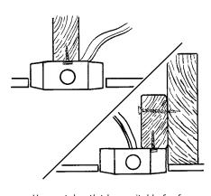
Use metal outlet box suitable for fan support. Secure outlet box directly to the building structure using ceiling joist screws (included). Junction box must support 35 lbs.
