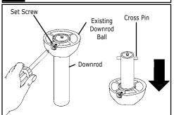
Remove the downrod ball that was supplied with your ceiling fan by loosening the set screw on the side of the ball so that it is no longer making contact with the downrod. Slide the downrod ball off
