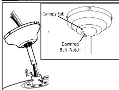
Feed motor lead wires through downrod/ canopy assembly and insert downrod into motor yoke. Make sure that the tab in the canopy engages the notch in the downrod
