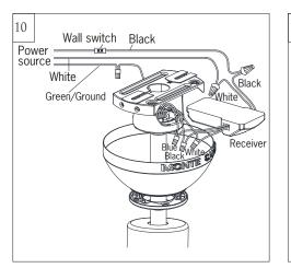
Make wiring connections using wire connectors provided as indicated above. White from fan to White from remote marked to motor N. Black from fan to Black from remote marked to motor L. Blue from fan to Blue from remote marked FOR LIGHT. White (Neutral) from house to White from remote marked AC IN N. Black (Live) from house to Black from remote marked AC IN L. Connect all green grounded wires to Grounded wire from House. Make sure that no filaments are outside of the wire connectors.
