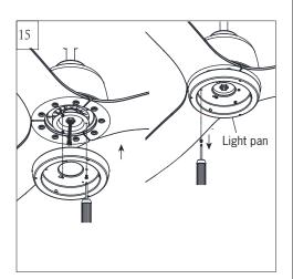
Place the lead wires from fan over the central hole of light pan. Aligning the keyhole slots on the light pan with the preassembled screws on the plate. Twist clockwise till lock. Reinstall the screw which was just removed. Tighten all screws securely. Loosen 2 and remove 1 preassembled screws from light pan. Keep screw.
