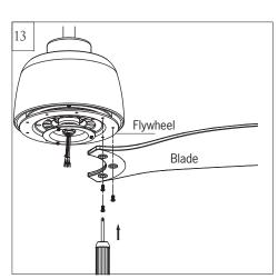
Install a blade onto the flywheel. Align the holes on the blade and the screw holes on the flywheel and install it with screws provided. Repeat this process for remaining blades. Tighten all screws securely.
