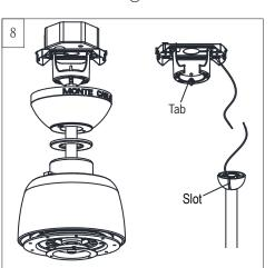
Install ball end of downrod into mounting bracket opening. Align (engage) slot on ball with tab on mounting bracket. **Warning:** Failure to align slot on ball with tab may result in serious injury. **Important:** If using the angle mount, make sure open end of mounting bracket is installed facing the higher point of the ceiling and make sure the ceiling angle is not steeper than 20°. Longer downrod may be necessary allowing the fan blades to rotate without obstructions.
